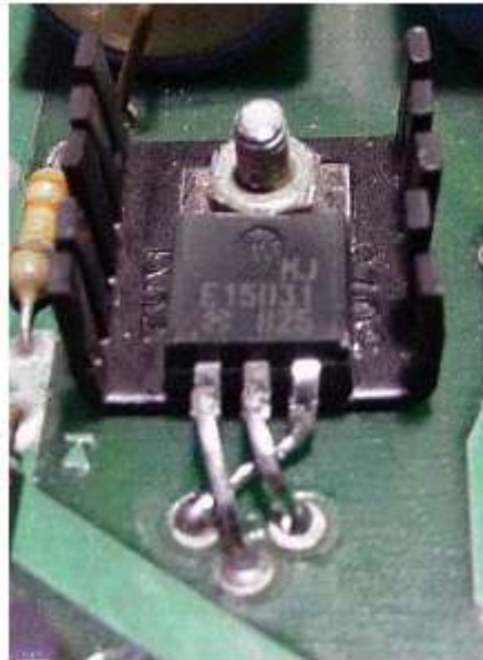
A replacement MJE15031 in an older System6 power supply:
