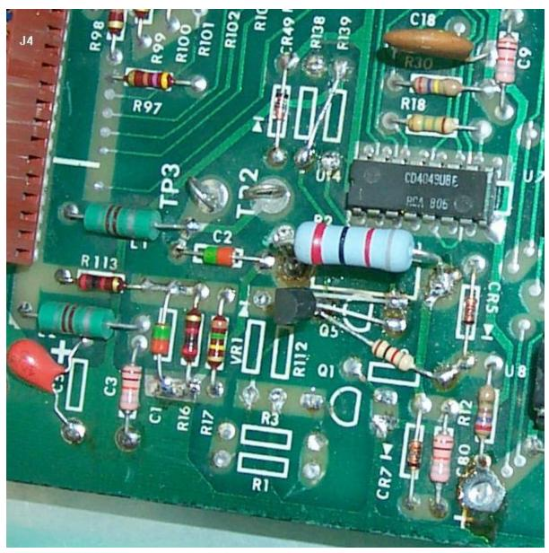
Note the 1k pull-up resistor is needed for additional current draw for all devices needing reset. If not installed, the MPU board can be intermittent on powerup because the DS1811 can't source enough current to bring the reset signal high by itself.
